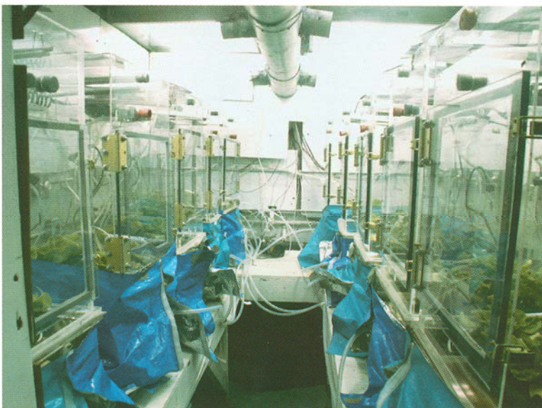
Plate 1–1. Photograph of the 10-chamber gas exchange system with independent hydroponic tubs.
